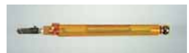
31 281 00 NIKKEN-Glasschneider NC-X02 Carbide-Schneidrädchen, schmal Schneidwinkel 138°, für 2-6 mm Glas NIKKEN glass cutter NC-X02 Carbide wheel, small cutting angle 138°, for 2-6 mm glass
